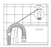
Place the discharging hose in a washbasin or sink with the aid of the bent piece delivered separately. The bent piece has to be entered into the tube's mouth in order to assure the support. Aforesaid piece allows the hose to be fixed to the wall by means of an opening on the upper part and that way the hose does not move and its falling is avoided.
